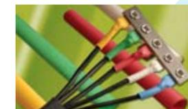
create a moisture proof seal blocking the entry of acids, gas, oil, and salt water. For environments with temperature extremes such as motor wells, irradiated polyolefin shrinkable tubing recovers to 50% of the provided diameter within seconds when heat is applied. It offers reliable protection and has an operating temperature range of -55°C to +130°C.
